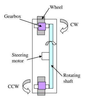
Figure 8: Rotating Shaft Steering Mechanism
