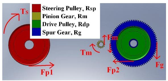
Figure 15: Free Body Diagram of Gears and Pulleys
