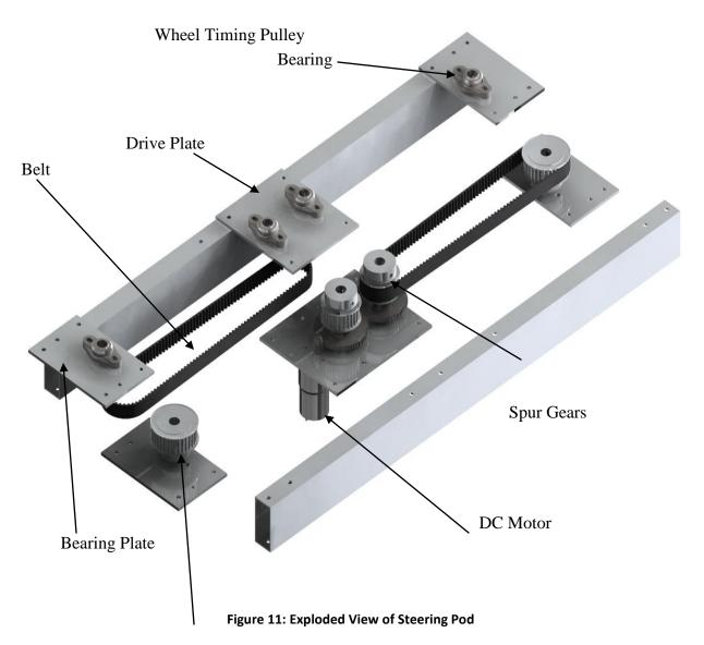
The motor is connected to the two spur gears. The motor serves to provide torque for steering. The two spur gears serve to create two opposing torques. Connected to spur gear by shaft, the drive timing pulley will then transmit the torque to the timing belt which will then transmit to the wheel timing pulley. Using this method, we are able to produce same torque with different direction at both ends of the steering pod.
