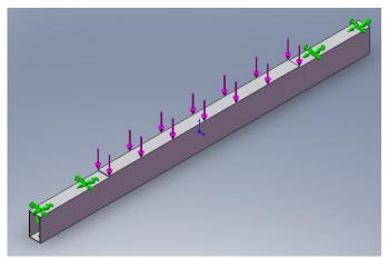
Figure 18: Boundary Conditions for Cross Beam
