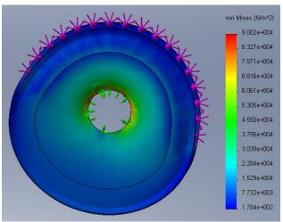
Figure 22: Pulley's Stress Distribution Plot
