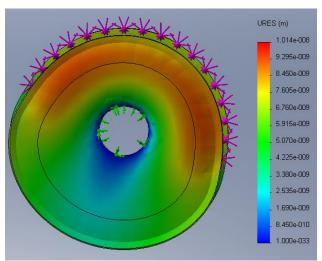
Figure 23: Pulley's Deformation Plot
