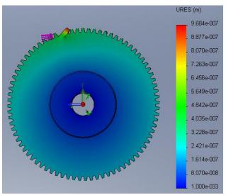
Figure 21: Displacement of the Spur Gear
