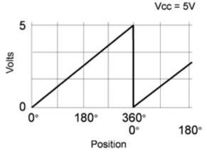
Figure 24: Encoder Output Voltage vs. Position
