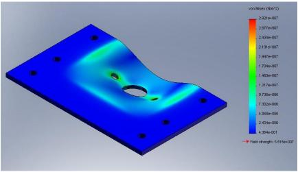
Figure 17: Stress Distribution on the Bearing Plate
