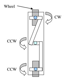
Figure 7: Linkage Bar Steering Mechanism
