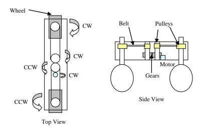
Figure 9: Gears, Pulleys and Belts Steering Mechanism
