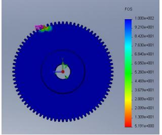
Figure 20: Factor of Safety of the Spur Gear
