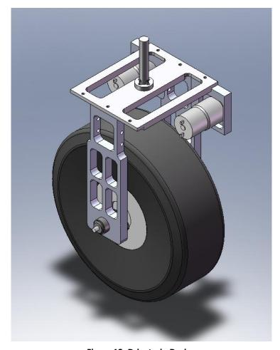
Figure 12: Drivetrain Design From SolidWorks, the resulting moment of inertia is:  $0.0104 \text{ kg/m}^3 + 0.0028 \text{ kg/m}^3 + 0.0002 \text{ kg/m}^3 = 0.0134 \text{ kg/m}^3$
