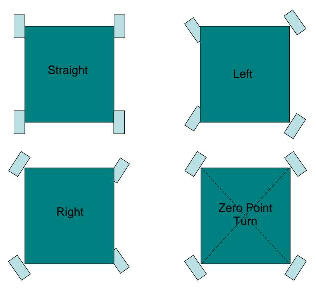
Figure 6: Configurations for different turnings
